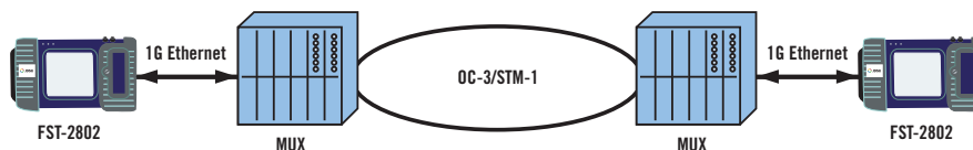
Diagram 1: Class of service testing using the Multiple Streams option for the FST-2802
